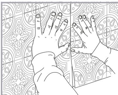
When the first panel is in place and you are happy that it's straight, line up the pattern on the next panel and repeat the process. Don't overlap the panels, make sure they are butt joined. Trim away any excess with your scalpel blade.
