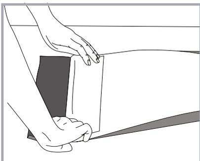
Peel away a 15cm section of backing paper and begin to smooth the panel on to the wall horizontally, lining the edge up with your plumb line. If you make a mistake, peel back and re-apply. Any air bubbles can be pushed out to the edges using your cloth or smoother.
