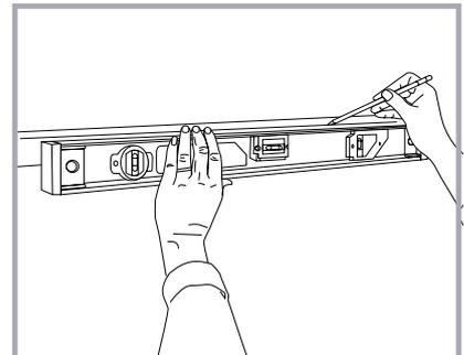
Using a spirit level, mark a horizontal plumb line on the wall as a guide to ensure you hang the panel straight.
